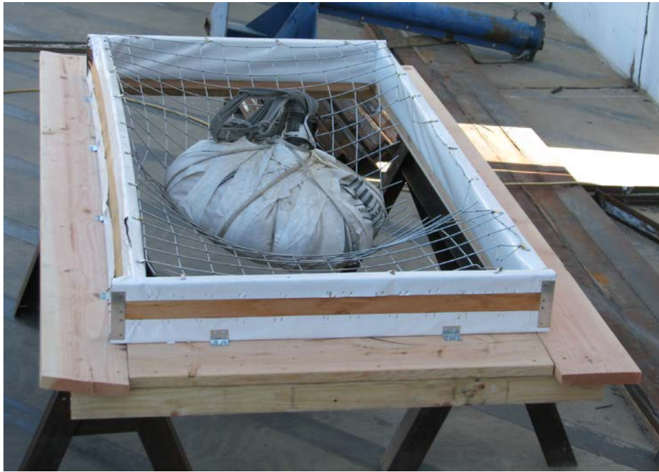
Photo No. 2 After impact, screen is holding test weight
