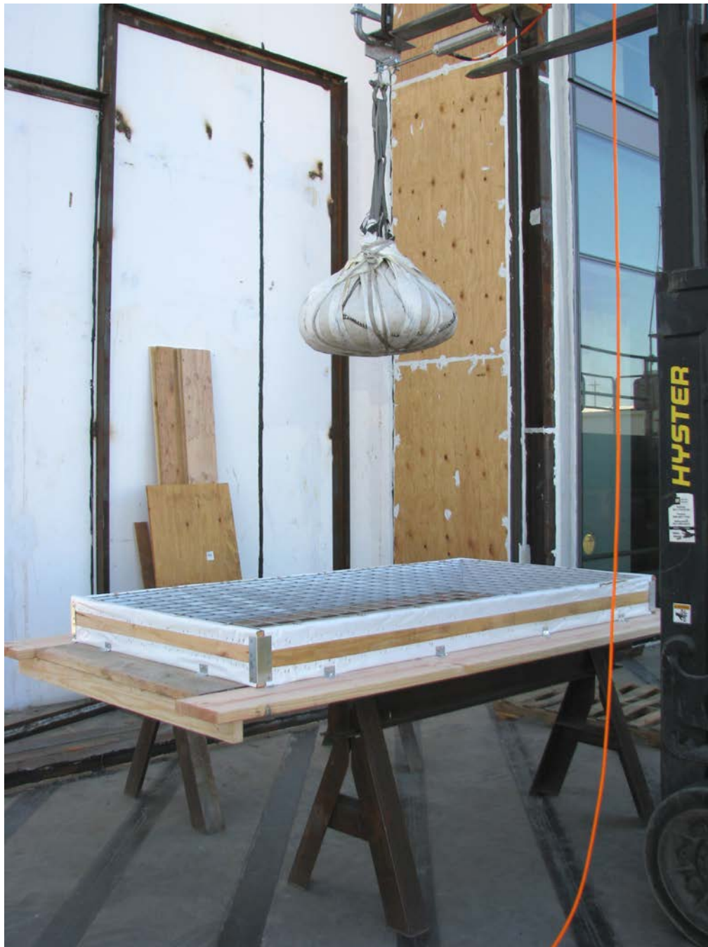
Photo No. 1 Drop test setup, test weight at 42" above screen
